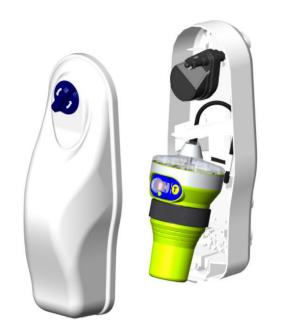
To mount the EPIRB in the category I bracket, insert the top cap first at a slight angle and then press the bottom casing until the EPIRB clicks and is firmly supported. The EPIRB can only be mounted inside the bracket with the ON/Test buttons facing out.
